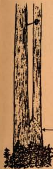
"DOUBLE SPAR" TREE WITH CABLING
